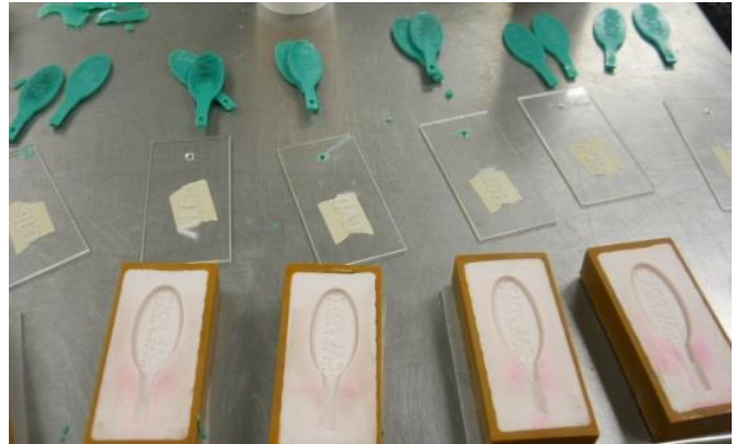
Figure 18) Injection Dies, Wax Patterns
