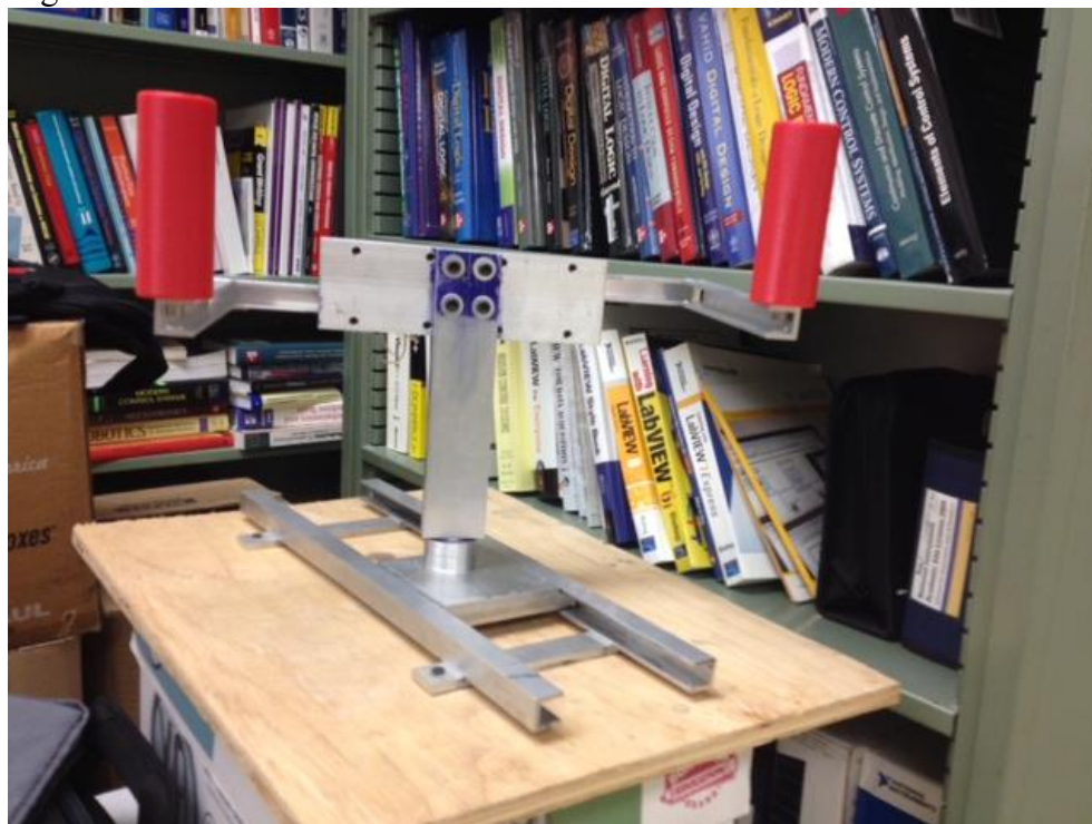
Figure 2. Mechanical Prototype for the Bimanual Rehabilitation Robotic Device.
