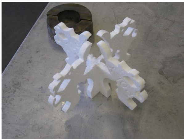
Figure 15) Foam Pattern Assembly
