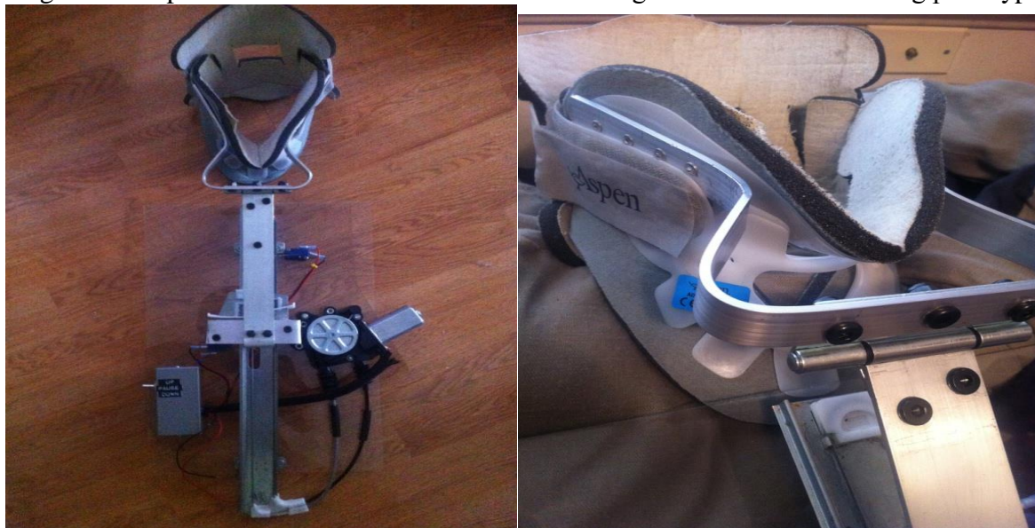
Figure 3. Motorized Neck Brace Prototype
