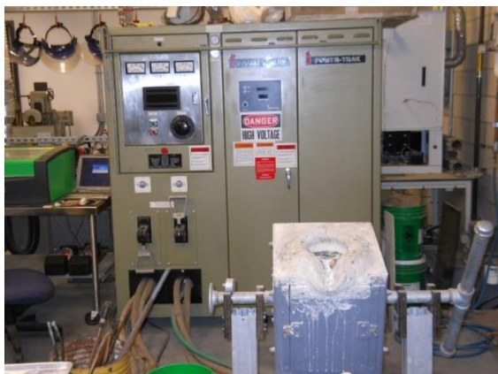
Figure 1) Induction melting system
