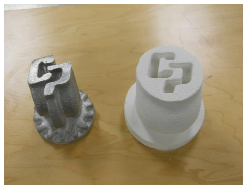
Figure 28) A 3D printer plaster mold and the casting
